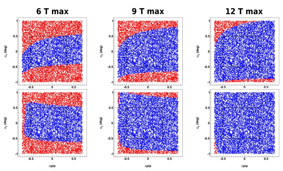
**Red**: Detection between the small upstream dipole and ion quadrupoles **Blue**: Detection after the large downstream dipole
